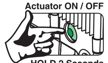
Figure 2: Powering ON the actuator
